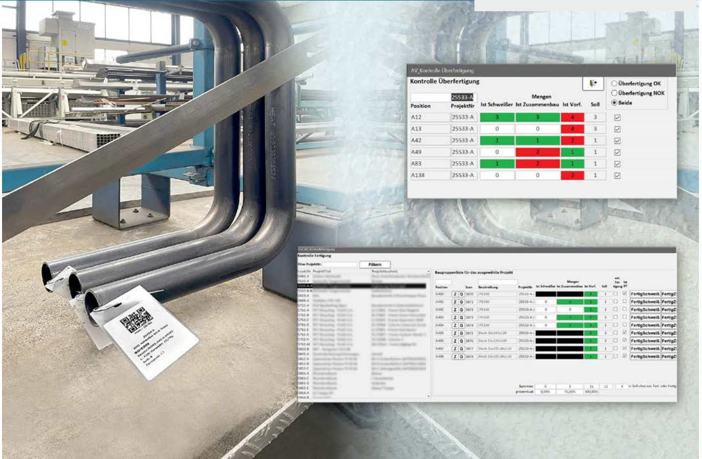
Figure 2: QR code on the component and excerpt from the software for checking and monitoring construction progress
