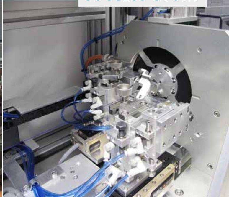
*heart of the machine: the yarn infeed and cutting*
