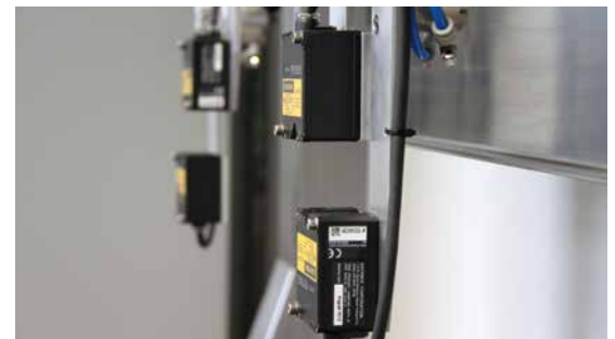
The laser measurement heads use the triangulation measurement procedure in order to determine the position of the reflected light on an RS-CMOS component. The position of the measurement object is measured by detection of the alteration of the way.
